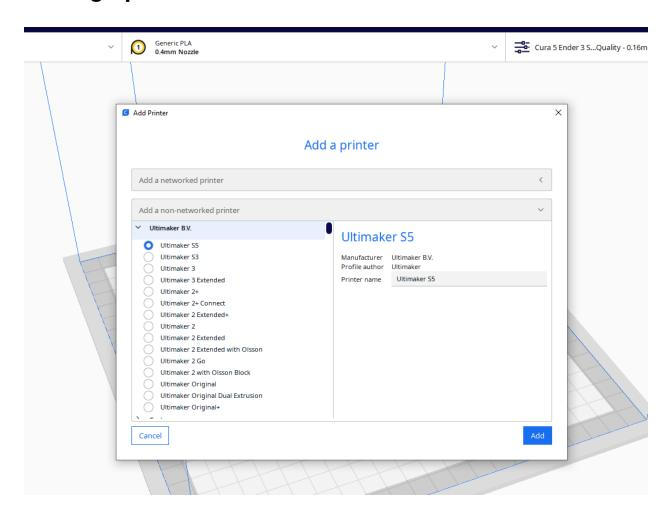
When you start Cura for the first time, it will take you through a walkthrough process to add your 3D printer. If not, go ahead and click on the 'Add Printer' option by the Folder icon in the top left, and select a 'Non-Networked' printer. Depending on your 3D printer, you may have to change additional options, as well as setting up the type of filament you would be using.
