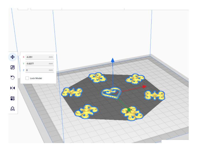
You can make minor adjustments to your model using the controls on the left. The most important ones are: Move, Scale, and Rotate.
