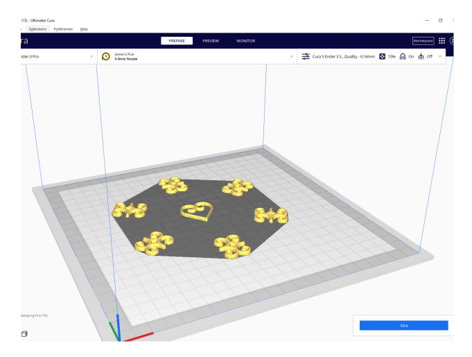
To import your model, go ahead and either drag and drop it into the software, or click on the File icon in the top left of the screen and select your model from your files. (I have imported a model created from the Adinkra Stamping software in this example).
