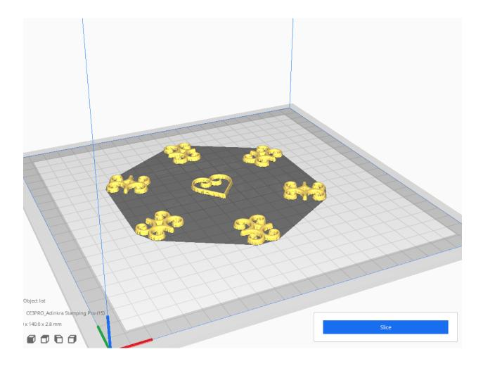
Once you are happy with your positioning and scaling, go ahead and hit **Slice.** This will generate the GCode (set of instructions) to use on the 3D printer. You can save it to a flash drive / SD card and plug it into your printer for printing, or send it via Wi-Fi depending on the type of printer you have.
