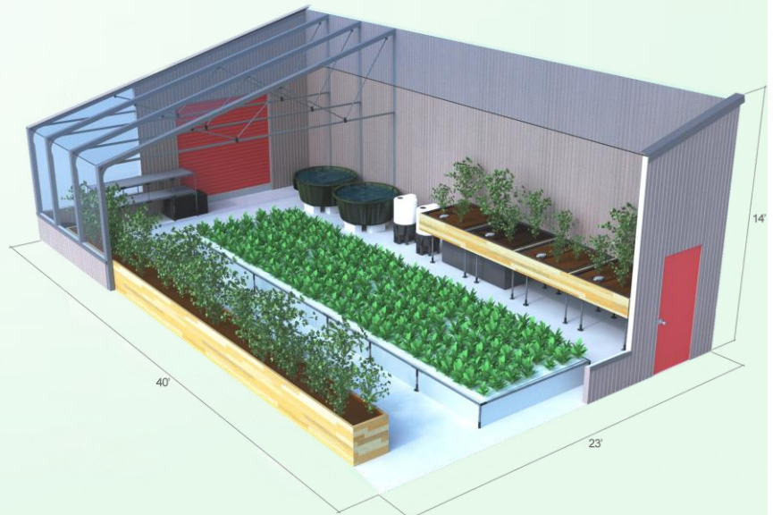
Rendering shows the Flourish 23' x 40' Aquaponic Farm in a Ceres Passive Solar Greenhouse with an east - west ridge line.
