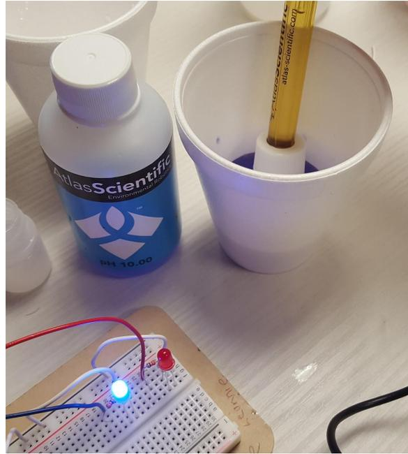
Image on the left is the result of placing the pH probe in the 4.00 pH calibration liquid (the red one) and the right is the result of placing the pH probe in the 10.00 pH calibration liquid (the blue one).
