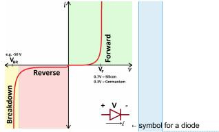
There are three important parts of this graph which are highlighted: forward, reverse, and breakdown. Based on the voltage applied, the diode will work differently.
